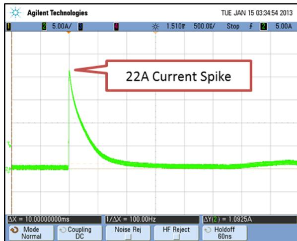
The waveform on the left illustrates the large current spike generated by “hot plugging” a module into a powered driver. This module normally requires approximately 10VDC to operate at 700mA. With no load, the driver defaulted to its maximum 48VDC output. During the initial contact between the driver and module, a current spike of 22A was generated! This type of stress can lead to premature failure of the module.
