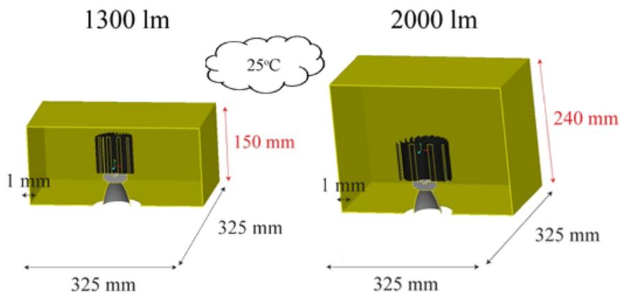
Figure 4 – Dimensions for successful enclosures at their minimum height in  $25^{\circ}\text{C}$  ambient
