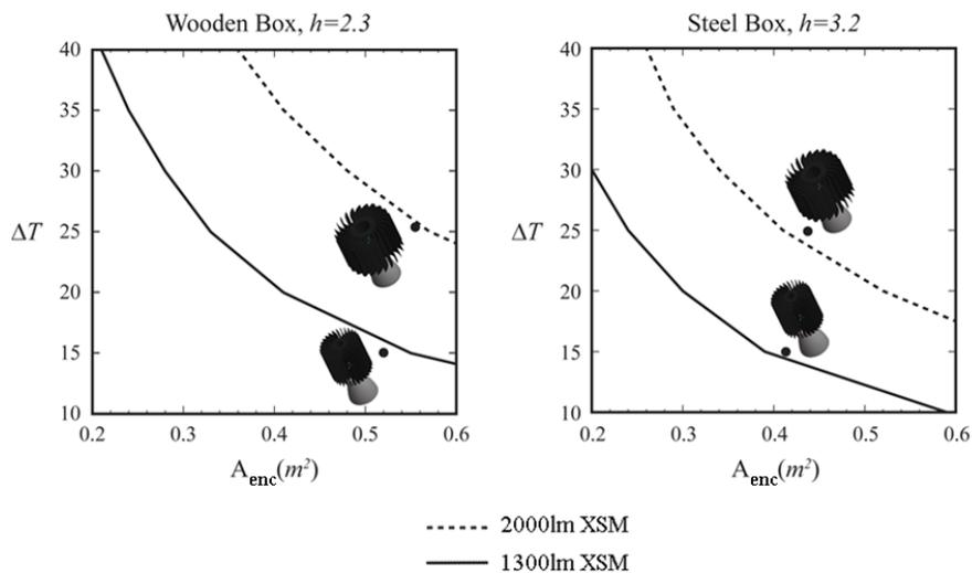
Figure 5 – Plot of Equation 1 for different XSM and enclosure conditions. The data points are results from the previous simulations.
