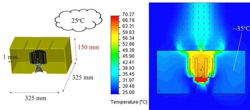
Figure 6 – 2000lm XSM in small enclosure with venting
