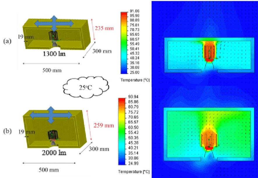
Figure 3 – Simulations of a 1300lm XSM (a) and 2000lm XSM (b) in a wooden box with rectangular footprint. Minimum height is determined for the maximum case temperature limit.
