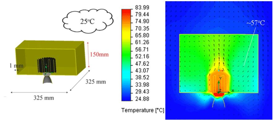
Figure 7 – Demonstrating the utility of using the enclosure as a heatsink
