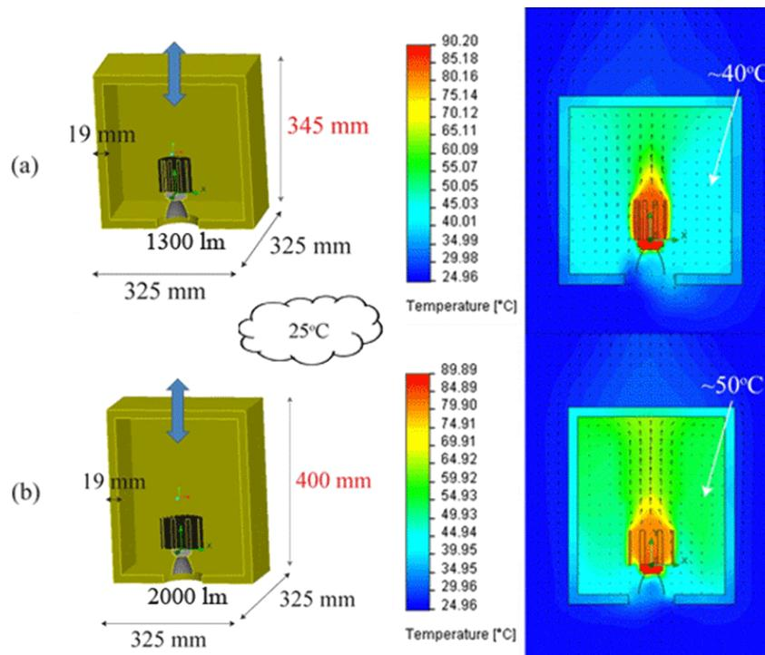
Figure 2 – Simulations of a 1300lm XSM (a) and 2000lm XSM (b) in a wooden box with square footprint. Minimum height is determined for the maximum case temperature limit.
