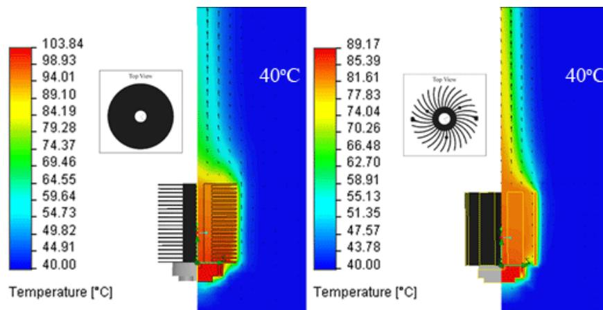
Figure 1 – Demonstrating the importance of heatsink design on case temperature
