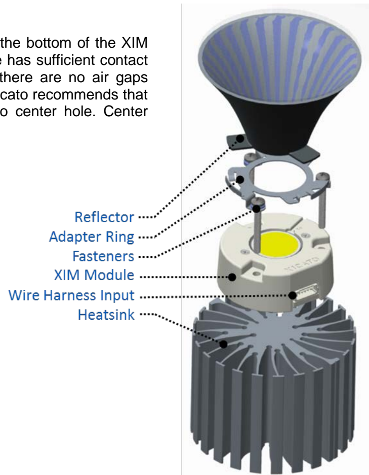
Figure 2: XIM Assembly (Exploded View)
