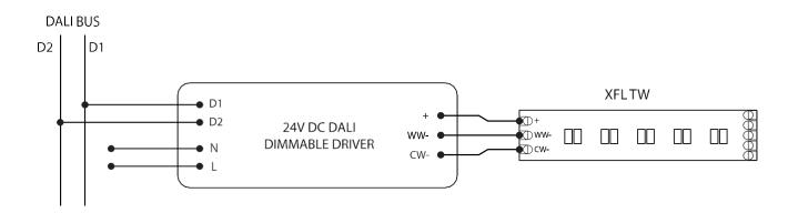
Wired + Wireless Wiring Diagram
